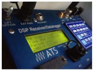
ATS receiver showing the inter-pulse period that is used to calculate the bat's temperature.
