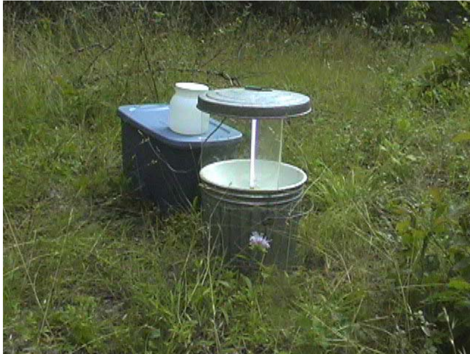
Figure 4.7. Illustration of the Ground black-light trap used to sample insects (23 June 2001).
