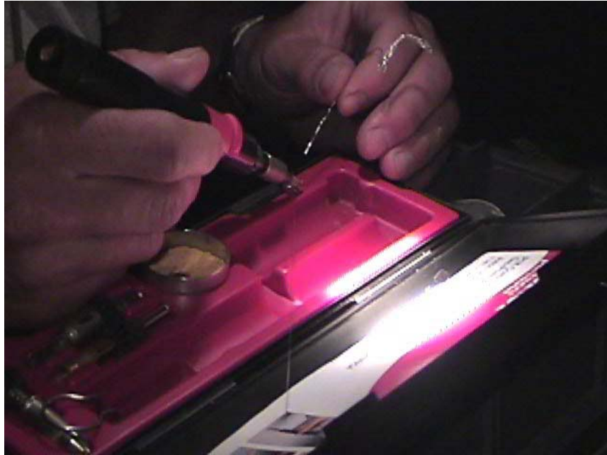
Figure 3.5. Illustration transmitter preparation, i.e., soldering power wires and applying surgical glue (Photo Taken 18 May 2002).
