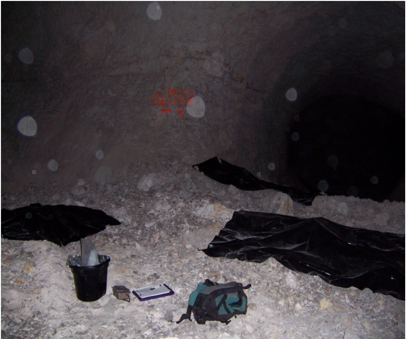
Figure 2. Picture showing the typical set-up of the plastic sheets in the rooms used in this study of the abandoned mines in southern Illinois from September 2006 through December 2007.
