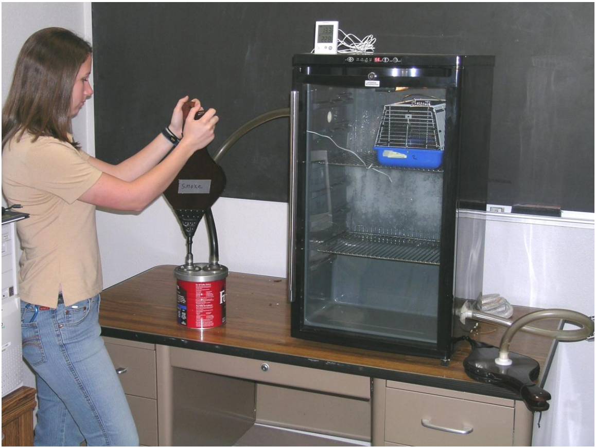
Figure 2. Smoke being added to the environmental chamber via bellows.
