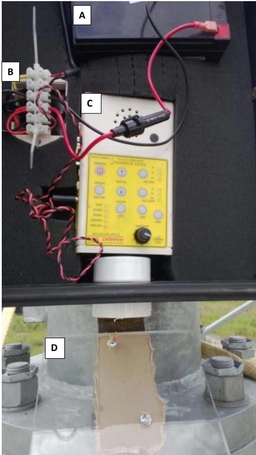
**Figure II.6:** Anabat SD2 (Titley Electronics) passive-acoustic setup placed six meters high on a tower leg. A) 12-V battery B) Solar Controller C) Anabat SD2, and D) Bounce plate. The bounce plate allows for reflection of calls into the microphone of the detector.
